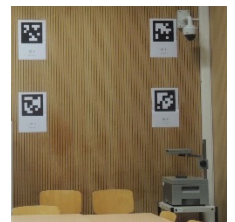
QR code to delineate zones for automatic analysis of elements captured by eyetracking glasses
